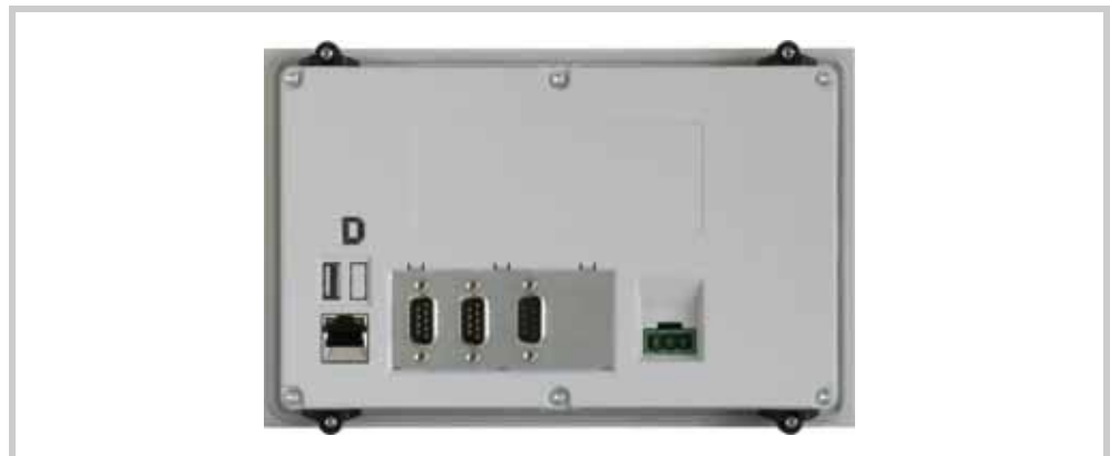
Fig.. 36 7.0" devices with four retaining brackets (do not meet IP65 / NEMA 4X requirements)
