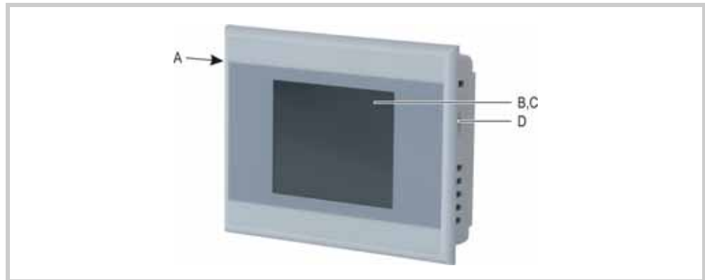
Fig.. 5 Example Operating and indication elements of the 3.5" devices
