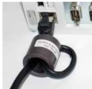
Fig.. 43 Ethernet cable, double loop through ferrite
